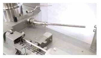
Stuffing of Large Diameter Product By installing straight stuffing tube, stuffing of large diameter product is possible.
