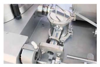
**Direct Piping** (with Magnetic filter) Without damaging meat, it is possible to produce high quality good taste sausage. Magnetic filter is optional device.
