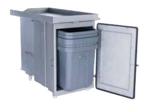
Peeled casings are delivered to the dust box in the vacuum tank. For customers who adopt central vacuuming system at their plants, we provide SABRE-20 without vacuum tank.
